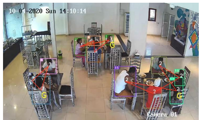
Fig. 12 Evaluation results of the retrained YOLO v3 model for detection of people. (Using both COCO person dataset and our custom person dataset)
