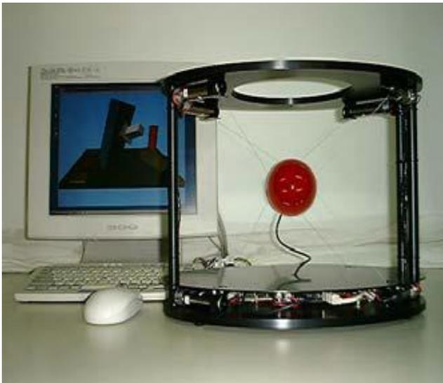
Fig. 1. SPIDAR-G haptic device
