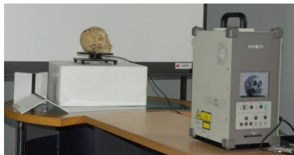
Fig. 10. The setup of acquiring the 3D model of the skull with the Vivid 910 3D Laser scanner at University of Colombo
