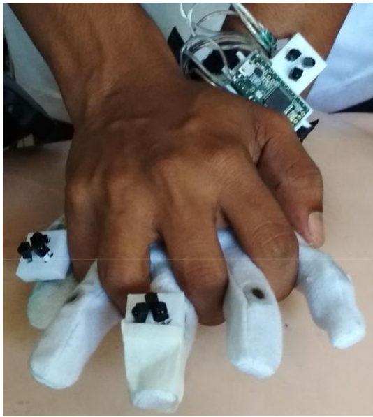
Fig. 6 Glove with three photodiode circuits
