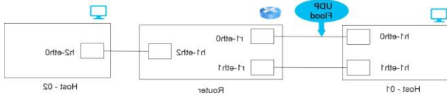
Figure 12: Test Bed on Mininet with UDP Flooding
